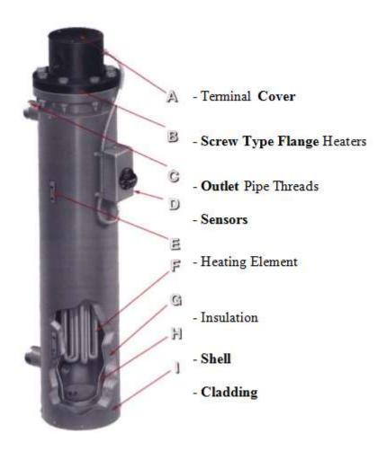
Circulation heaters are the most common types of electric heaters used in the process industries. Tubular elements are welded into a flange to form the heater. One of the most important criteria for designing an immersion heater or a circulation heater is to choose the proper watt density of the heating elements. The liquid, gas, or solid that you are heating must have the correct watt density to ensure that the heater is safe, properly sized, and have a long life.
